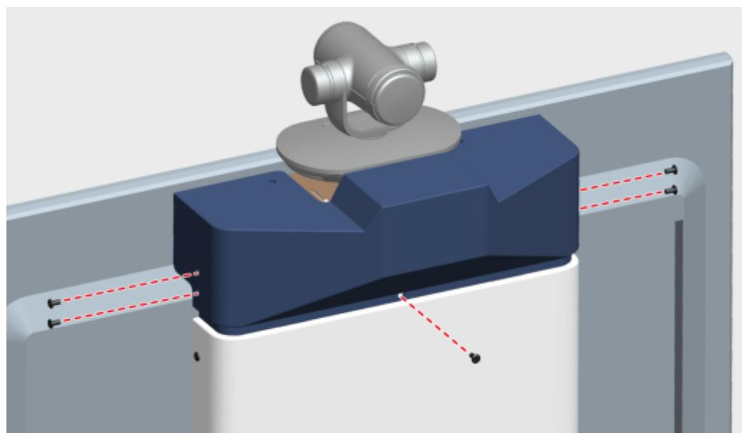
**Step 11** Fasten the TE30 composite cable.
