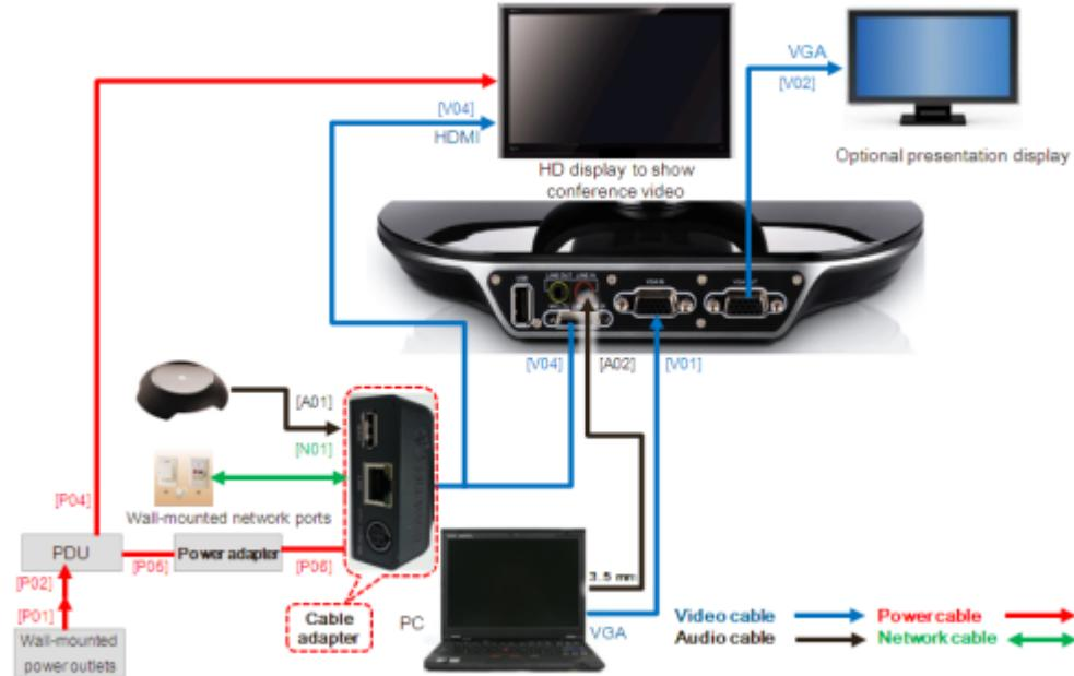
Figure 4-5 RP200-46S/55S cabling
