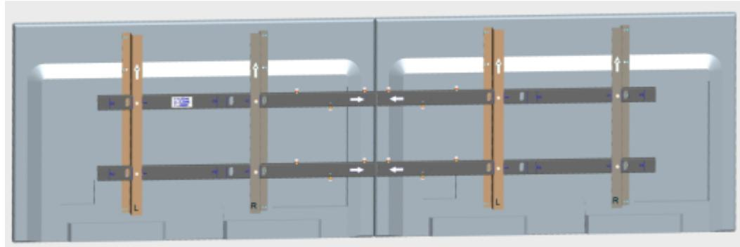
**Step 7** Align the HD display holes with the holes silk-screened with the number that matches the HD display model on the L and R bars, as shown in Figure 3-24.
