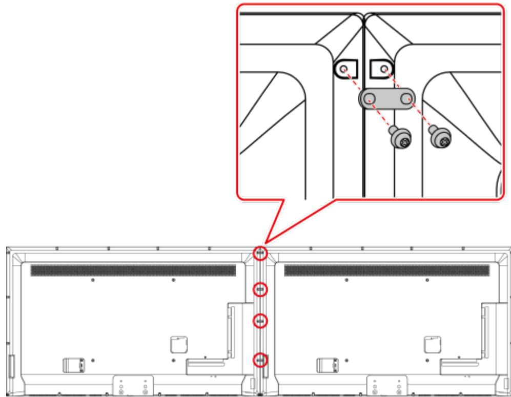
**Step 6** Keep the arrows on the horizontal bars facing inward and arrows on the L and R bars pointing towards the top of the HD displays. Place the supports on the rear of the HD displays, as shown in Figure 3-23.
