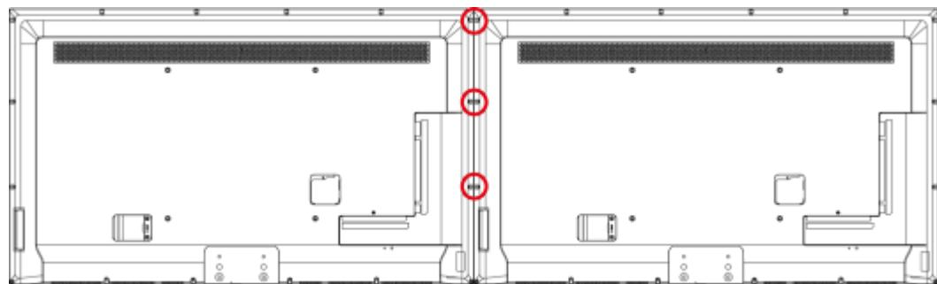
**Figure 3-20** Installation positions of the connecting plates for 55-inch HD displays
