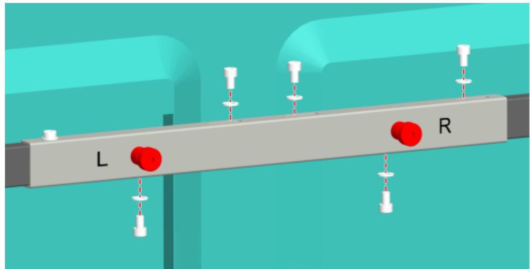
**Step 13** Ensure that the L and R bars are vertical to the horizontal bars; otherwise, move the horizontal bars to adjust.
