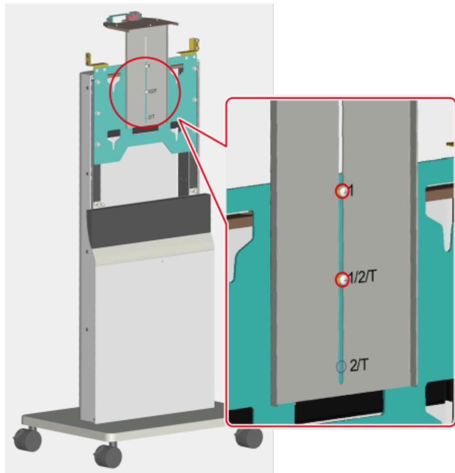
**Step 2** Tighten the screws using a Phillips screwdriver to secure the camera mounting bracket.
