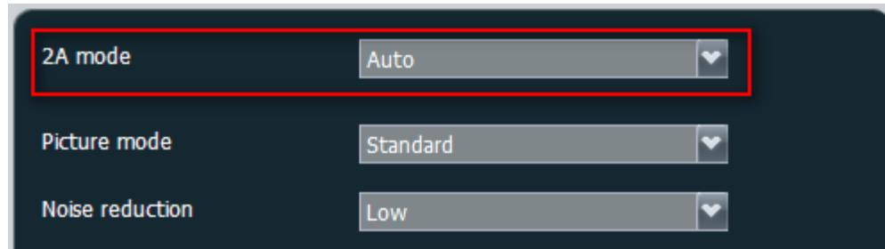
If the actual environment is tough and the camera brightness and color fail to meet requirements, set **2A mode** to **Manual** and adjust the other parameter settings for a satisfying effect.
