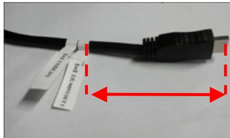
Some cables may have a ferrite bead close to the connector. In this case, the labels must not be attached between the connector and ferrite bead, as shown in Figure 4-3.
