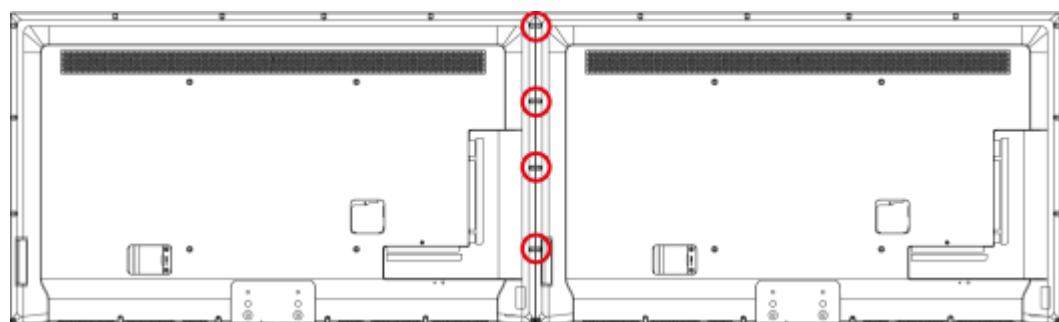
3. Fasten M3 x 12 recessed pan head screws in the holes where the screws were removed to securely attach the connecting plates, as shown in Figure 3-21 and Figure 3-22.
