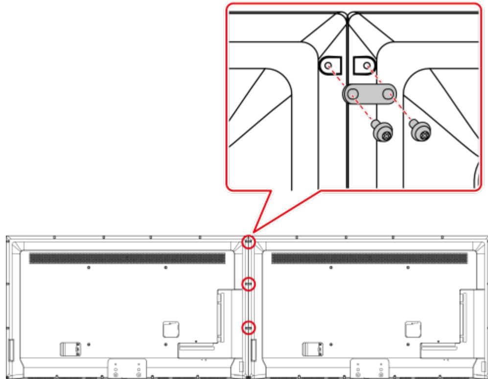
**Figure 3-22** Installing the connecting plates for 55-inch HD displays
