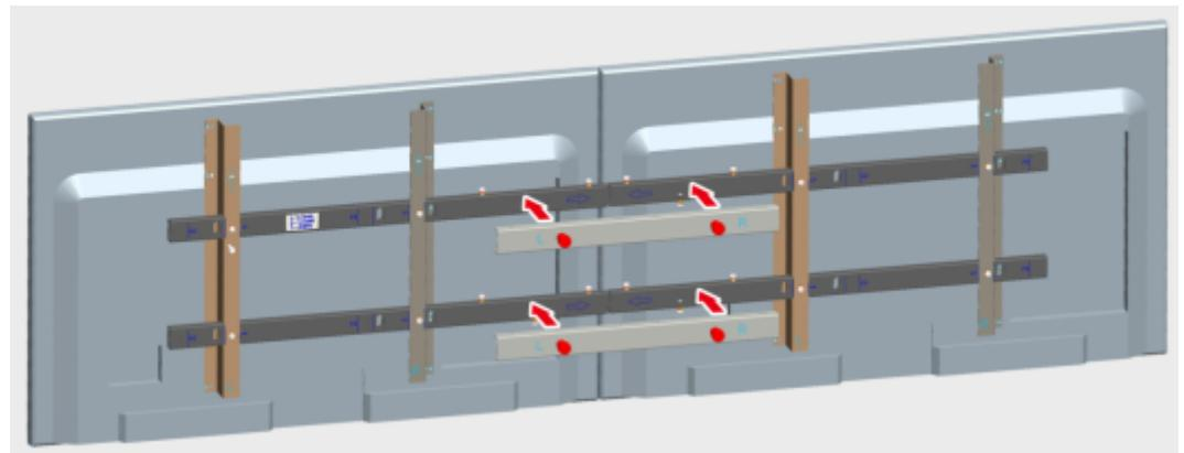
**Step 11** Align the holes on the connecting bar with the holes on the horizontal bars of the supports. Fasten the screws and washers, as shown in Figure 3-27.
